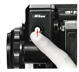
Keep depressing the chrome button and when the proper aperture for the selected shutter speed has been obtained, the sound stops and both signal lights glow. In the viewfinder you will see the selected aperture and shutter speed. When another combination is desired, reset the shutter speed and the attachment will adjust again for the right aperture.
