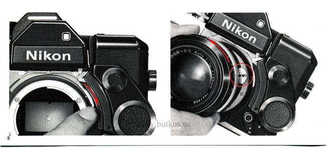
Turn the lens' aperture ring all the way to the minimum aperture setting, then all the way in the opposite direction. Check the maximum aperture indicator on the F2S Photomic Finder to make sure that the maximum aperture of the lens in use appears in the window. For example, if the 50 mm f/1.4 lens is mounted on the camera, the number 1.4 should appear in the window.
